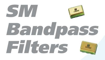
Utilizing DLI's high permittivity, COG/NPO ceramics allow for small size, temperature stable performance over frequency and high reliability in environmentally challenging conditions. This series of bandpass filters was designed to span the popular 1.22-28 GHz frequency range. The compact size and surface mount attachment allow for low cost of manufacturing without sacrificing performance and repeatability. Designed for use on PCB 8-12 mils thick with a permittivity of 3.0-3.8.
